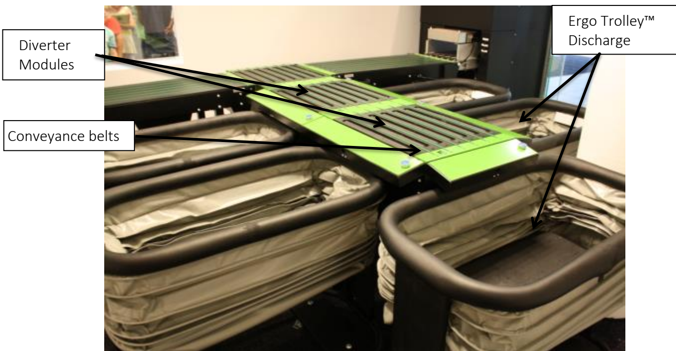
Figure 22- Sort Mate™ components
